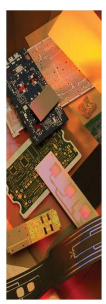
**51N** is a non-DICY multifunctional epoxy low-flow prepreg system designed to provide high reliability through lead-free solder operations. The high decomposition temperature and high thermal stability of this material is ideal for use in complex rigid-flex fabrication and assembly operations where minimum resin flow is required.
