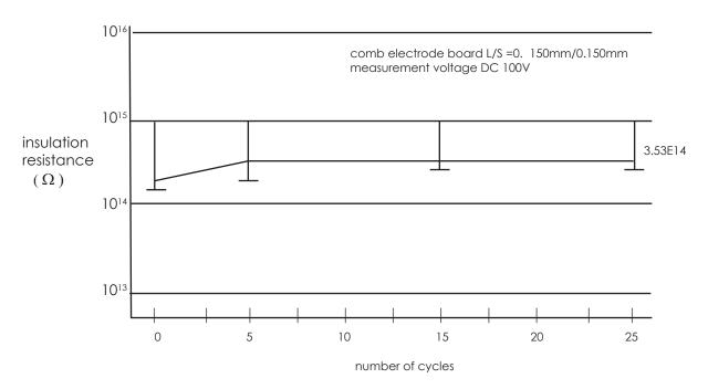
**Electrical Insulation characteristics**
