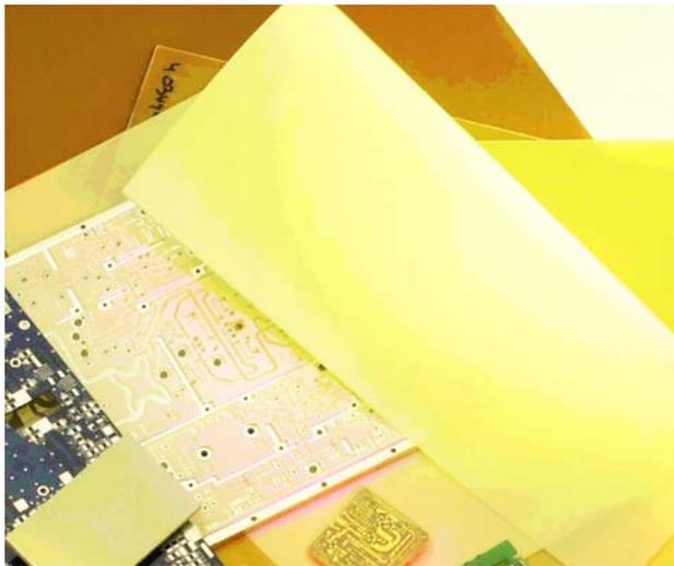
AD320A is a woven fiberglass reinforced PTFE/Microfine Ceramic composite material and is a significant improvement in cost/performance over traditional fluoropolymer-glass laminates that do not use ceramics. This combination offers designers an advantage for improving electrical performance through the use of advanced material without the additional cost traditionally associated with higher performance.
