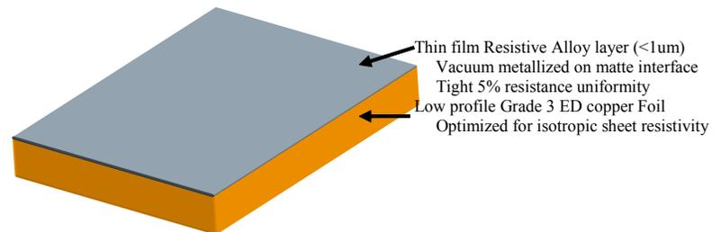
**Figure C – Formed Embedded Resistor**
